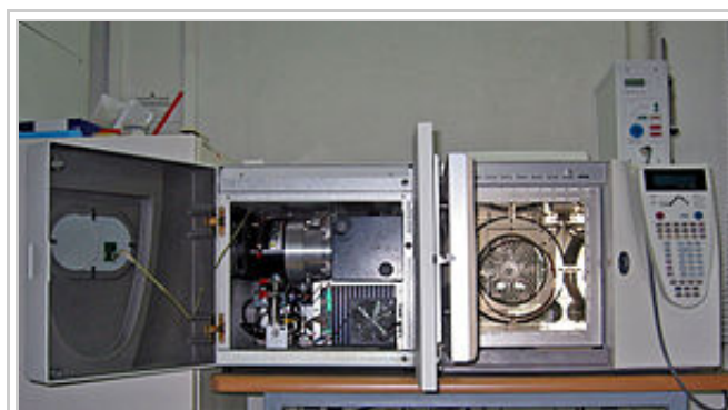
A gas chromatograph (right) directly coupled to a mass spectrometer (left)
