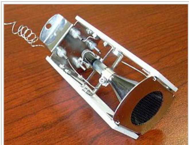
A continuous dynode particle multiplier detector.
