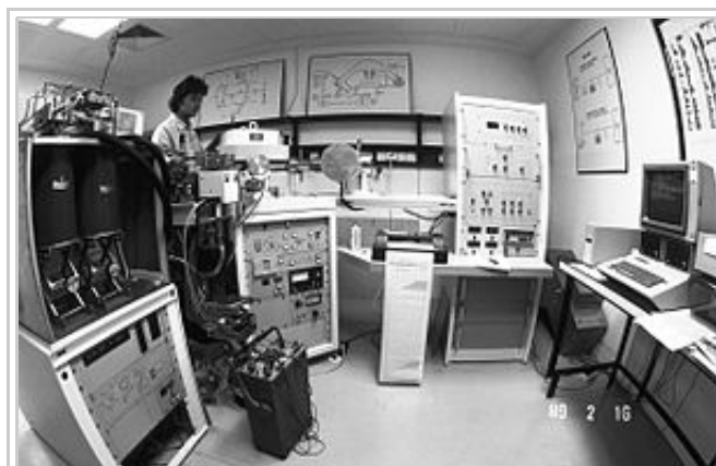
Mass spectrometer to determine the ^{16}\text{O}/^{18}\text{O} and ^{12}\text{C}/^{13}\text{C} isotope ratio on biogenous carbonate
