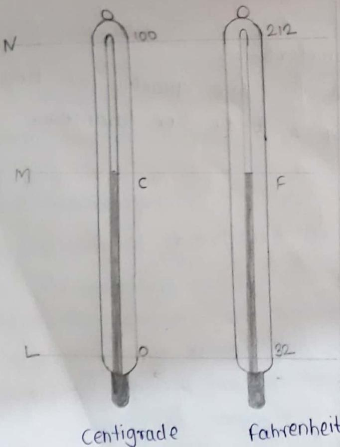
consider two identical thermometers marked in centigrade & fahrenheit scales. Place the two thermometers in a bath at certain fixed temperatures. Mercuray in each thermometers stands to the same level M. as shown in fig.
