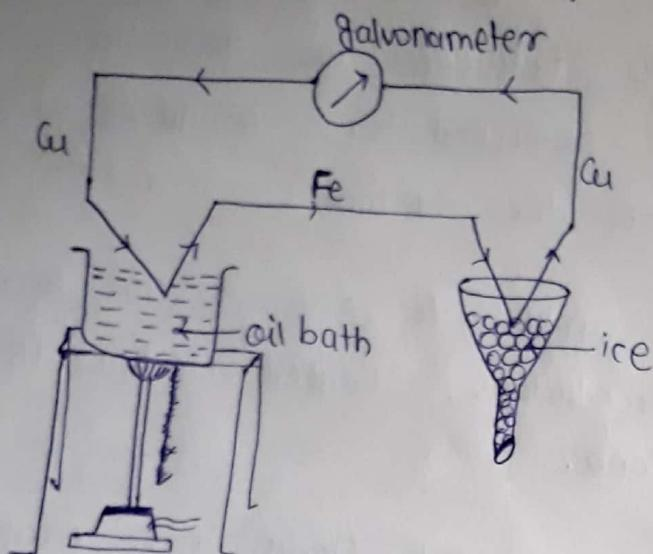
If both the junctions are at  $0^\circ\text{C}$ , there is no deflection in the galvanometer.
