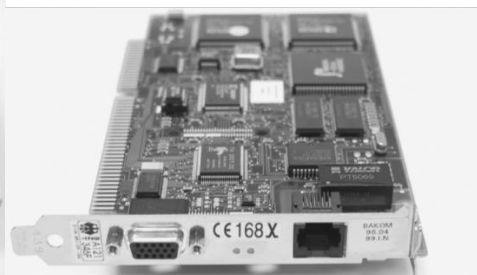
a) An External ISDN Adaptor b) An Internal ISDN Adaptor
