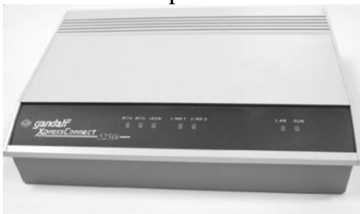
a) An External ISDN Adaptor b) An Internal ISDN Adaptor
