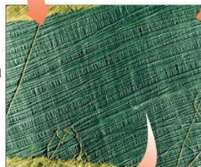
Fibers formed from aligned cellulose
