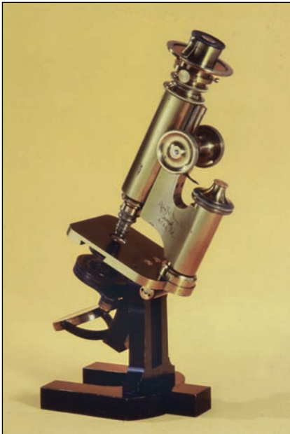
A 19th-century monocular microscope. These instruments were capable of high resolution but difficult to use for extended periods of time. (courtesy of the author)
