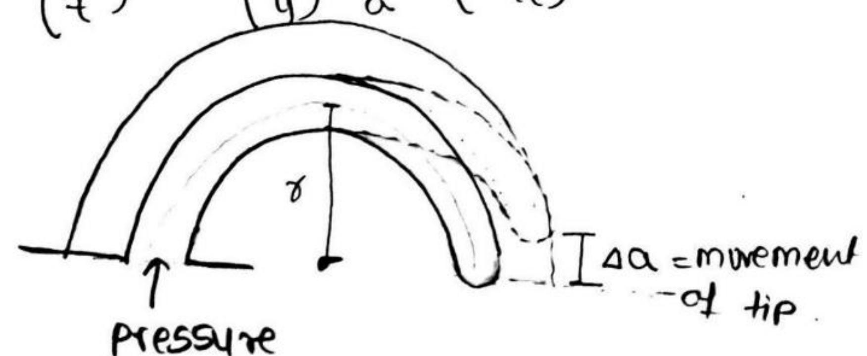
Thus, the relationship between the displacement of tip and the applied pressure is nonlinear ie each pressure increment does not produce a corresponding tip movement.
