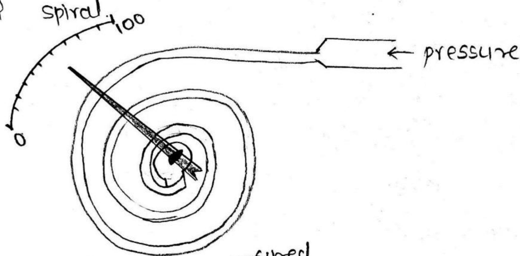
When the pressure <sup>to be measured</sup> is applied to the spiral, it tends to uncoil producing a relatively long movement of tip whose displacement can be used for indication.
