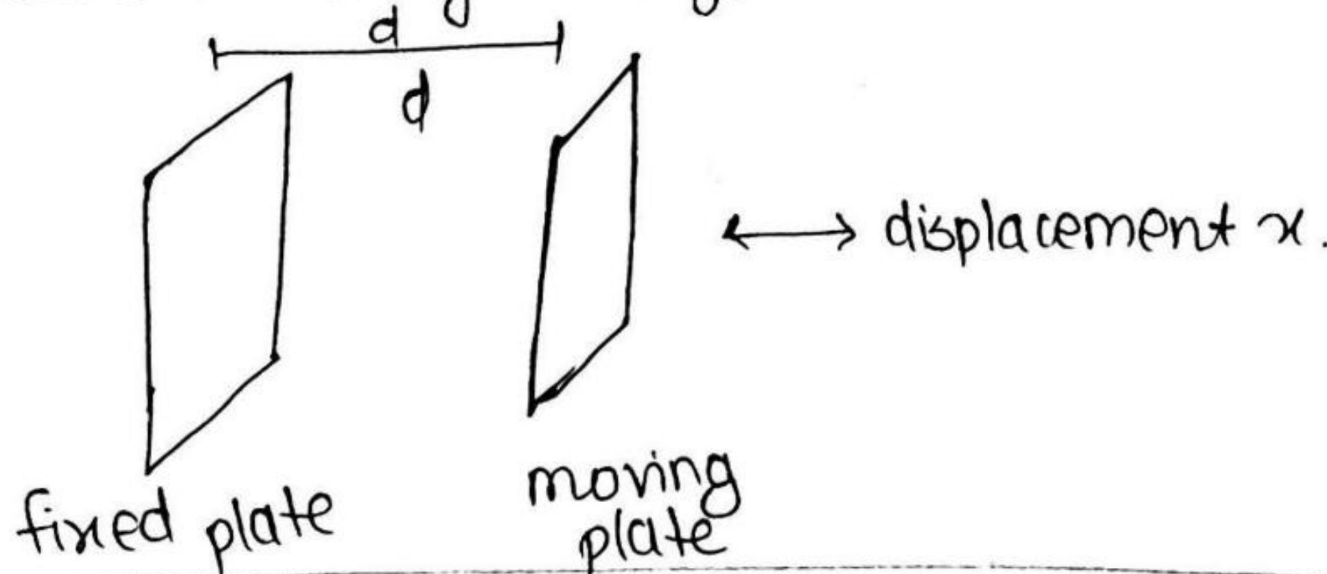
above diagram shows the basic form of a capacitive transducer utilizing the effect of change of capacitance with change in distance between the two plates. One plate is fixed and displacement to be measured is applied to the other plate which is movable.
