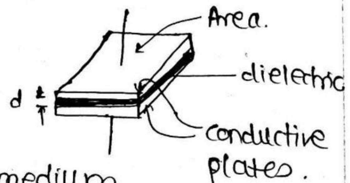
The ~~capacitor~~ capacitive transducer works on the principle of change of capacitance which may be caused by -
