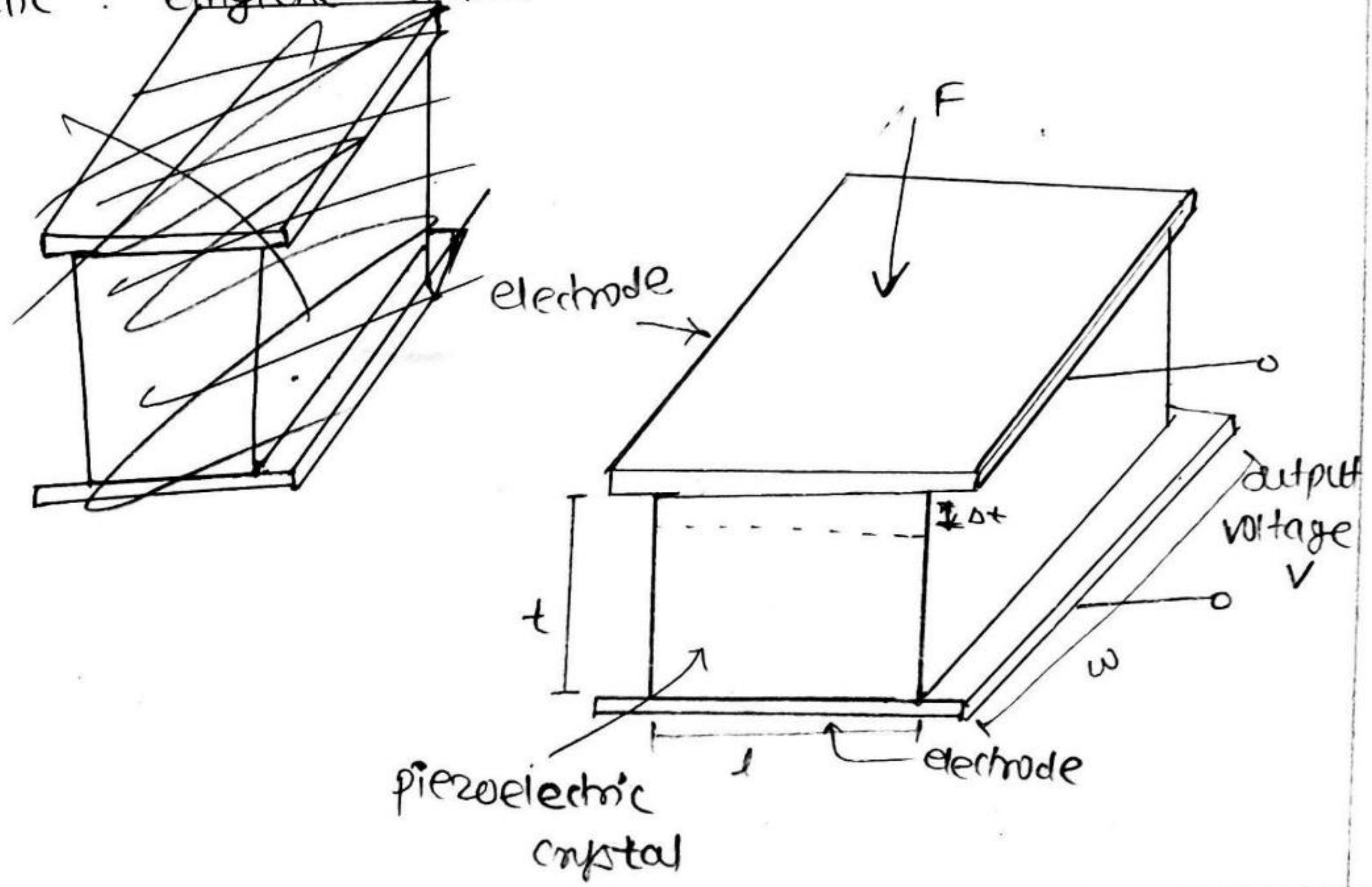
The charge  $\varphi$  is accumulated on the electrodes, when a force  $F$  is applied on a crystal and is given by
