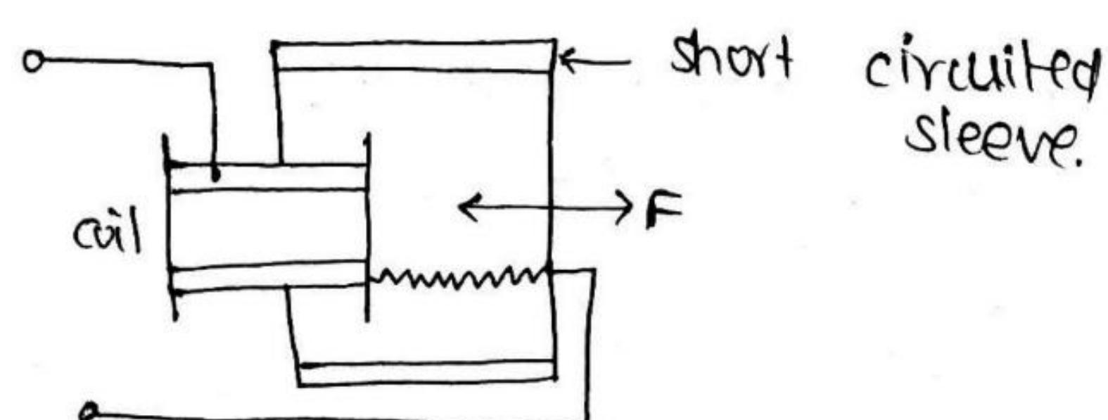
The plate may be at right angle to the axis of the coil. The displacement of plate causes a change in inductance of the coil.
