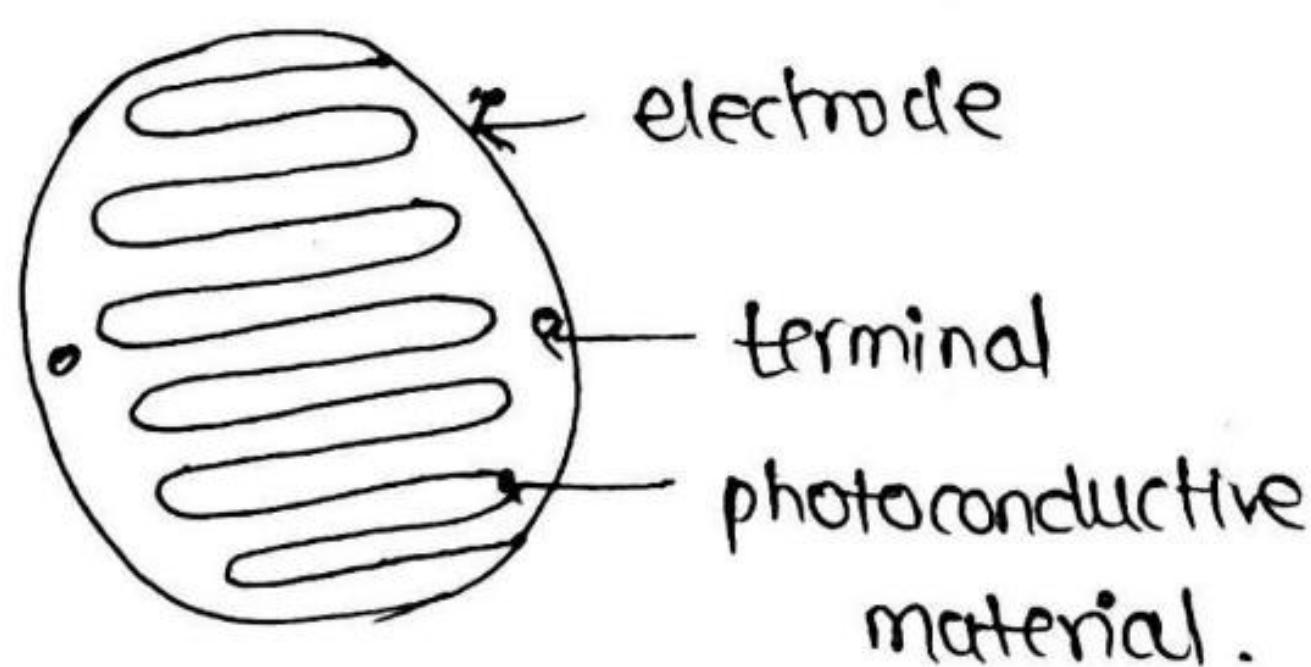
A photoconductive cell is as shown. It consists of a disc shaped base in which a long strip of a light sensitive material is placed in a zigzag pattern. On each side of the strip, connecting terminals are fitted. It is to be noted that the connecting terminals are <sup>not</sup> connected to the ends of the strip, rather they are fitted in the conductor on each side of the strip. This makes the light sensitive material appear to be a short and wide strip with conductors on both sides.
