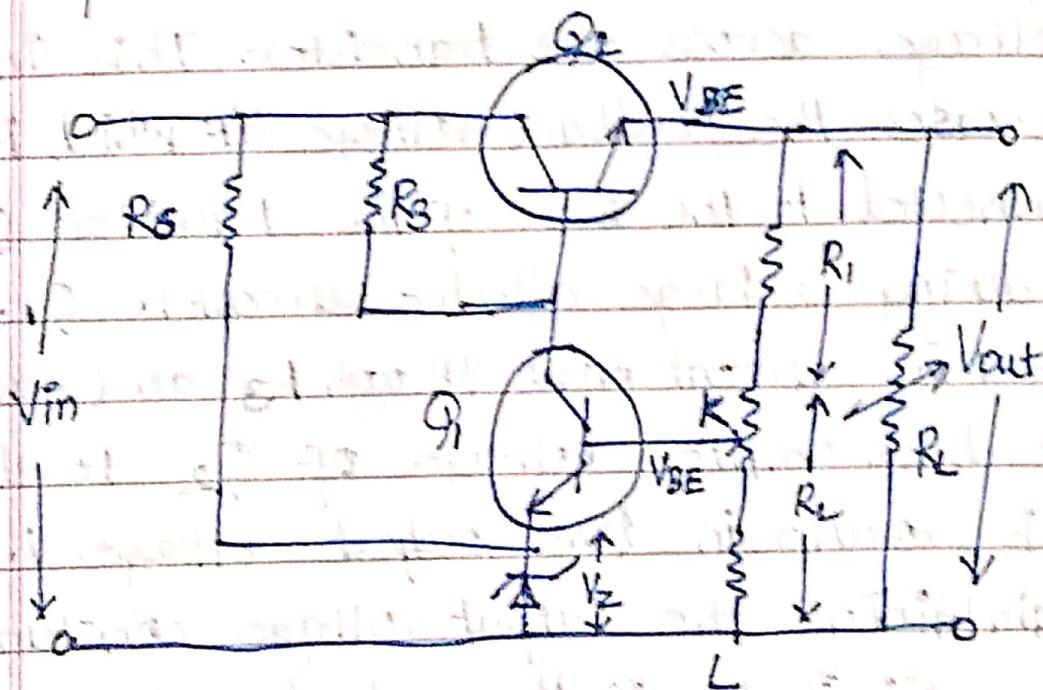
The transistor  $Q_2$  is called as pass transistor becaz all the load current passes through it. The circuit consist of voltage divider that consist of  $R_1$  &  $R_2$ . These act like the voltage dividers which supply the output voltage and gives it as a negative feedback voltage to the base of the transistor  $Q_1$ . The feedback voltage
