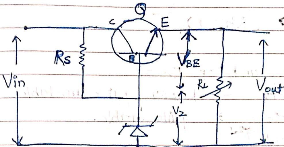
In the circuit, the base voltage of the transistor  $Q$  is held relatively constant across the Zener diode.
