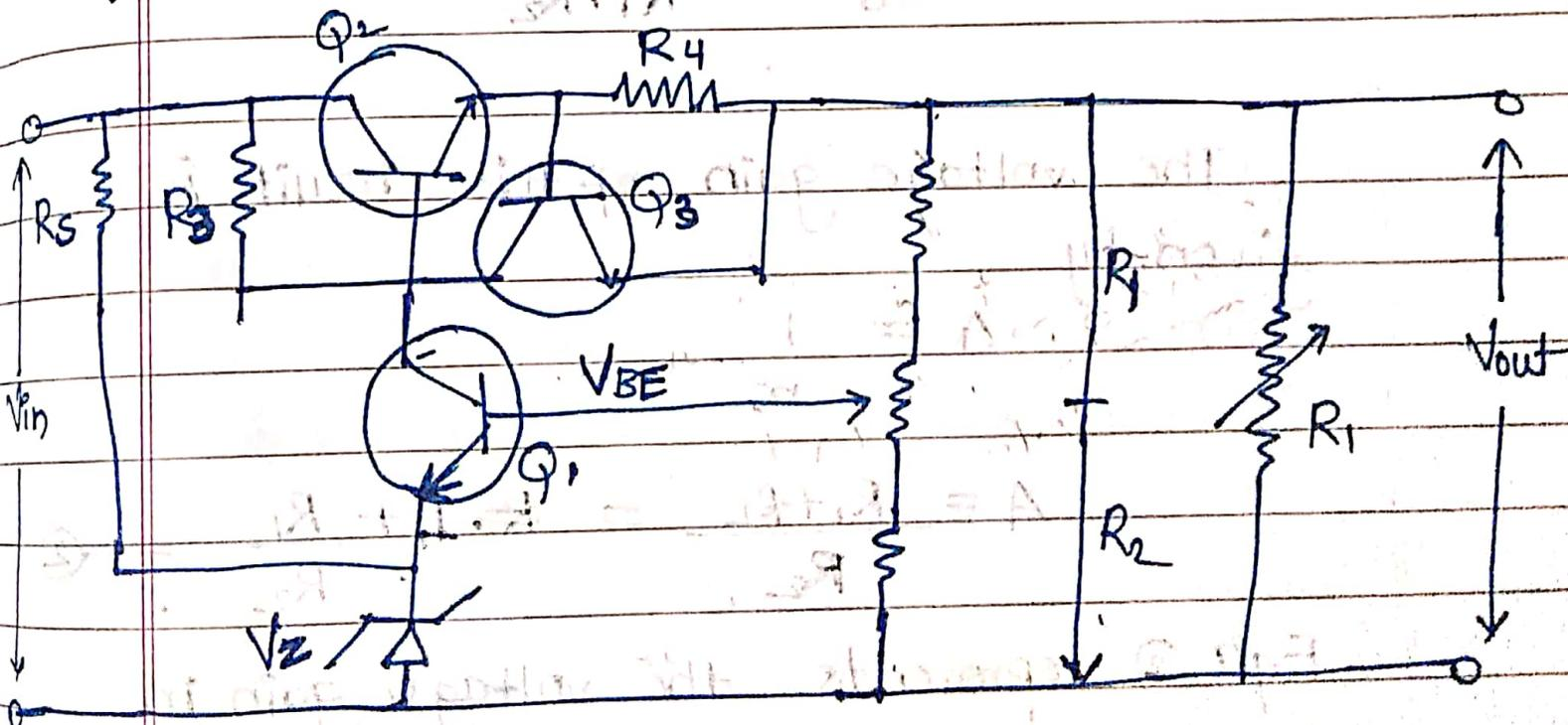
The transistor series feedback voltage regulator has only one drawback i.e. any series regulator can be destroyed by continuous excessive load current, if the load is shorted. To avoid this short circuit a current limiting circuit is added to series regulator. It consist of a transistor and a resistor.
